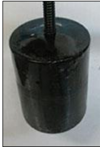
Figure 2: Response P™ after 22 days of exposure to 90°C in 3% KCl
