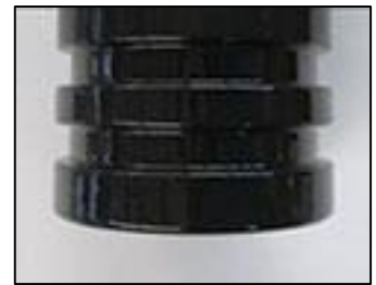
Figure 4: Response P™ after 30 hours in RT 15% HCl
